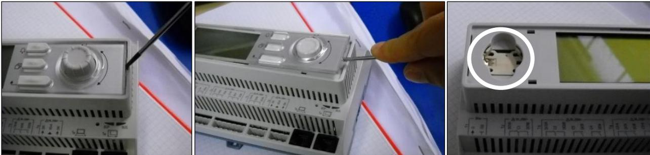
Be careful to avoid damages to the plastic cover. The new battery shall be placed in the proper battery holder which is highlighted in the picture, respecting the polarities indicated into the holder itself.
